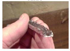
For the solder, I took one part lead to five parts tin (Theophilus pp56). I melted them together and used the lead came mold to form the solder (Photo G). As Theophilus described there is no reason to make a mold when you already have one.
