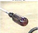
For one of the bladders I was allowed to blow on the blow pipe to get an idea of how much (or little) pressure was needed to blow air into the glass. The bladders we made went into the annealing chamber and, once again, they had to stay there overnight.
